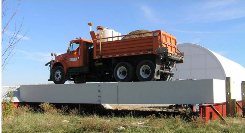
Figure 7. Gravel truck applying load at test site
